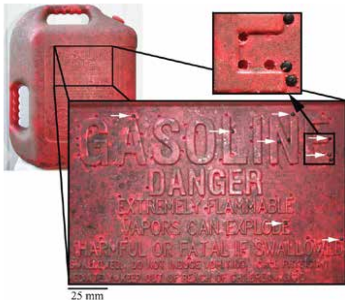
Damage to a gasoline container caused by female camphor shot borers (from Carlton and Bayless 2011, used with permission).
