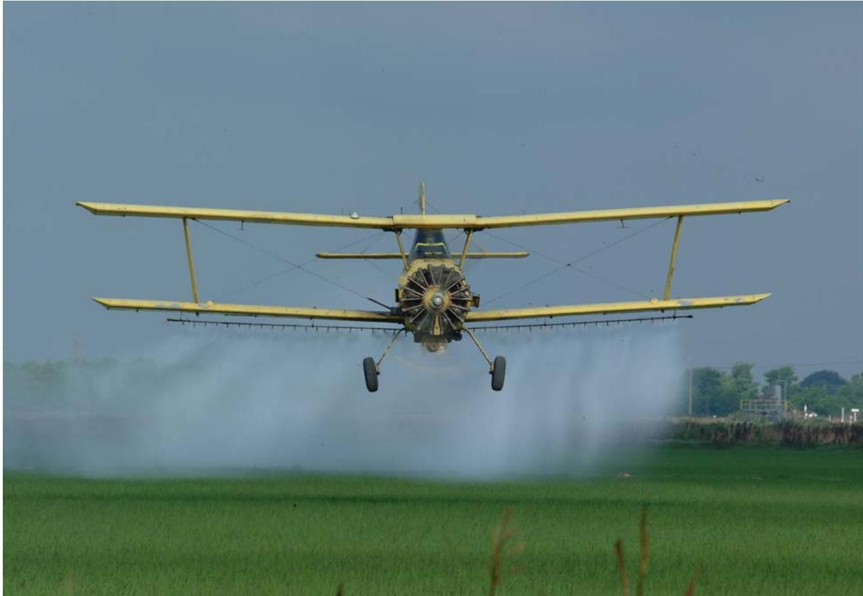
The aircraft shown above was applying Clincher herbicide to our verification field in Vermilion parish. The label states it should be applied at 10 gallons per acre. Based on what is visible here I think we got the appropriate amount. Don't call me about how lower rates work just as well, I've heard all of the arguments and understand the difficulty aerial applicators face in remaining profitable. We are following the label requirements.
