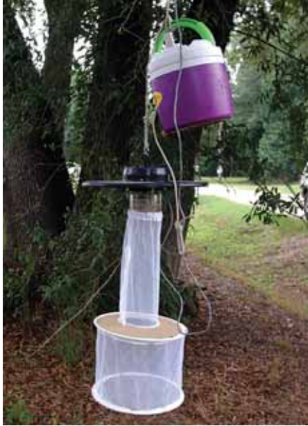
Figure 3: The CDC (for Centers for Disease Control) miniature light trap is typically hung from a tree and includes a light to attract flying mosquitoes and a fan to suck them into the white net tube. The cooler hanging next to the trap contains dry ice, which is carbon dioxide (CO 2 ) in a solid state. CO 2 attracts mosquitoes.
