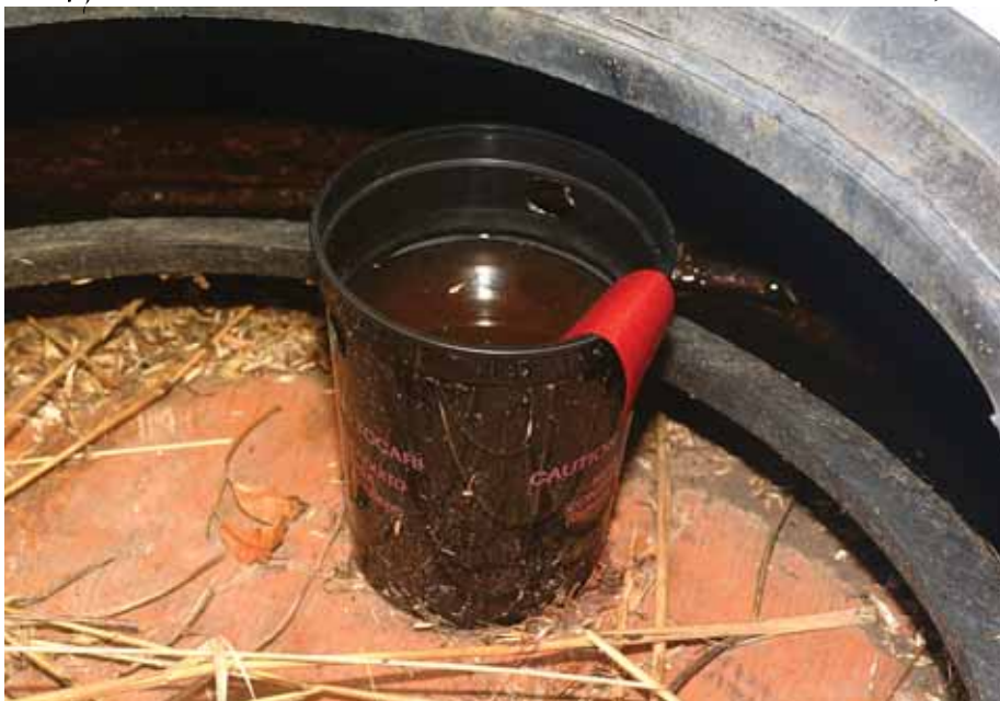
The ovitrap is placed in areas where there is standing water. It includes a black plastic cup half filled with water, with a wooden paddle or paper strip resting inside. The mosquito lays eggs on this strip.
