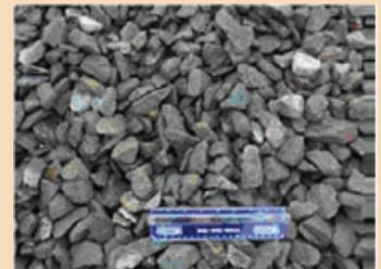
Figure 6. No. 4 crushed limestone.
