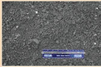
Figure 8. Densely graded aggregate for the surface layer.
