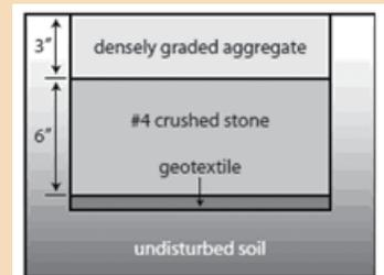
Figure 1. Construction details.
