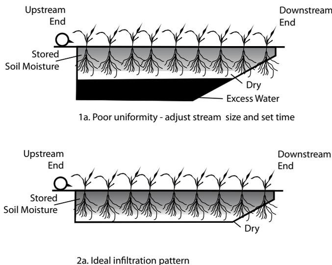
**Figure 1. Infiltration profiles under conventional furrow irrigation.**
