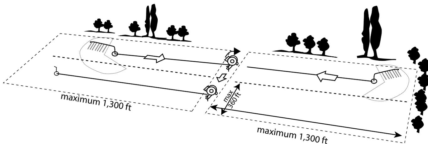
**Figure 2. Layout of a hard-hose drag traveler. Travel lanes are 100-360 feet apart, depending on sprinkler capacity and diameter coverage.**
