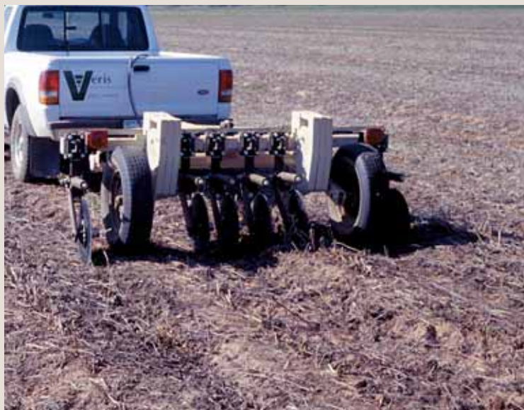
Figure 1. A Veris model 3100 sensor cart used to measure soil electrical conductivity at the Dean Lee Research Station. The unit is manufactured by Veris Technologies, a Division of Geoprobe Systems, in Salinas, Kans. The coulters on the outside of the wheels measured to 36-inch depths in this study. The coulters inside the wheels measured to a 12-inch depth.
