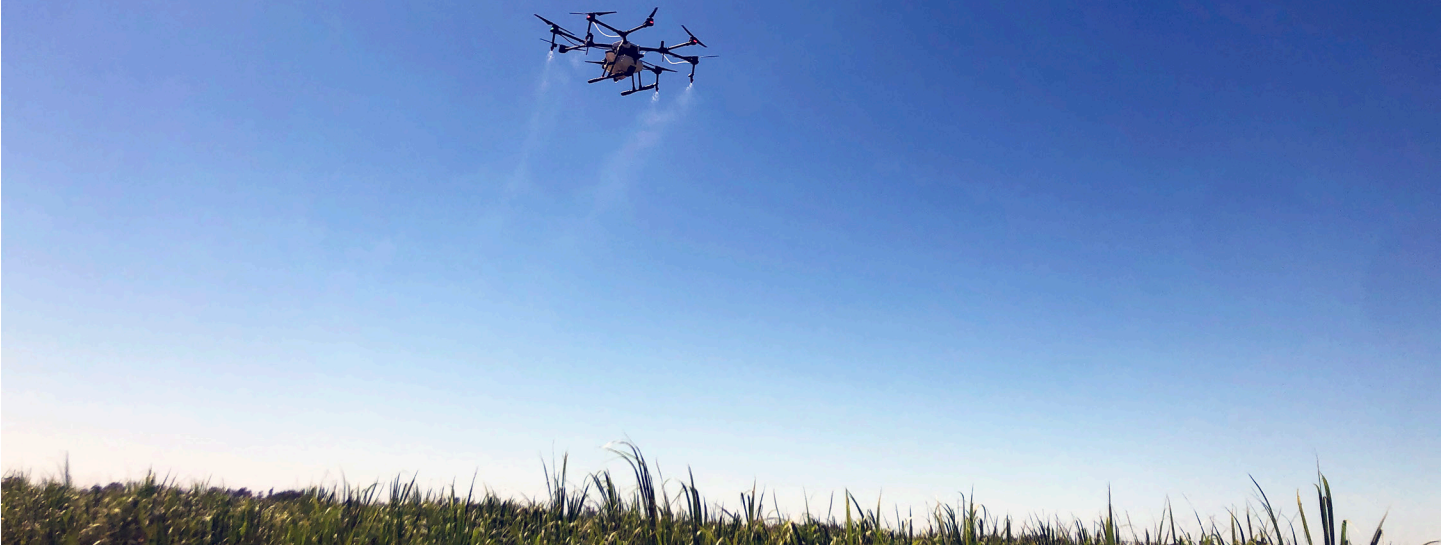
An agricultural spray drone applies ripener to sugarcane.
