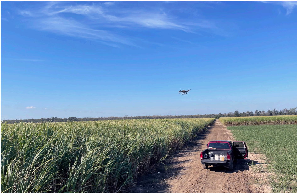
An agricultural spray drone applies ripener to sugarcane.
