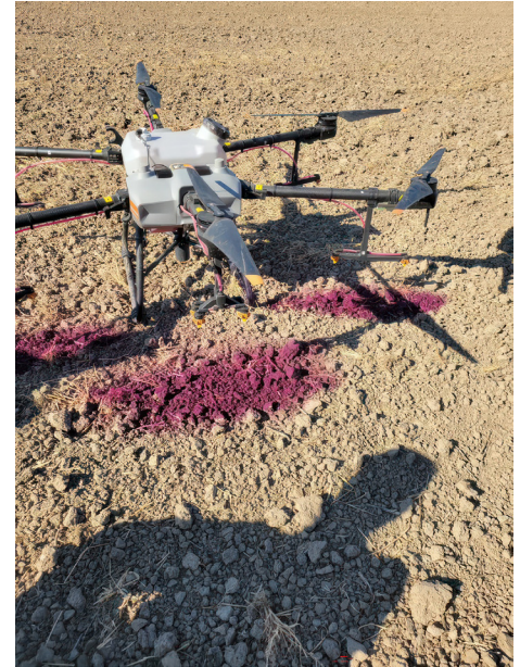
Drone with florescent dye sprayed on the soil.
