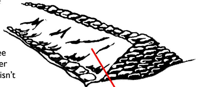
*This plastic reduces water seepage but is more vulnerable to damage from floating debris. Weaving plastic sheeting into the sandbag levee is better.*
