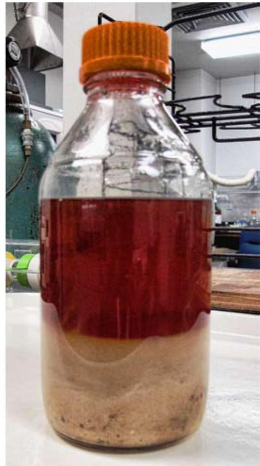
**Figure 3.** Sample collected from the bottom of a settling tank separates over time, depending on the ambient temperature.
