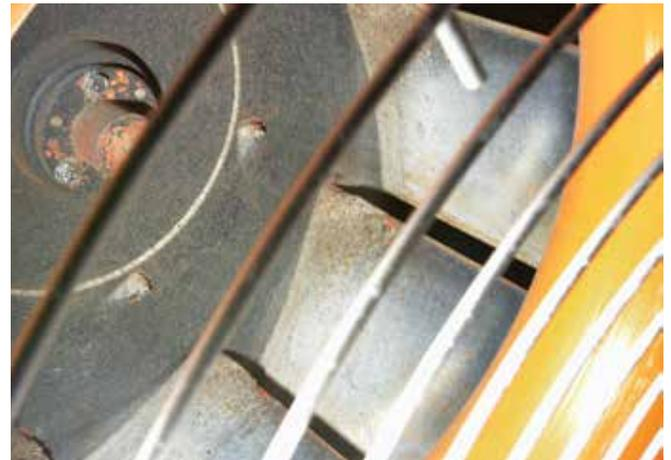
*Fig 8-3. Blades of centrifugal fan.*
