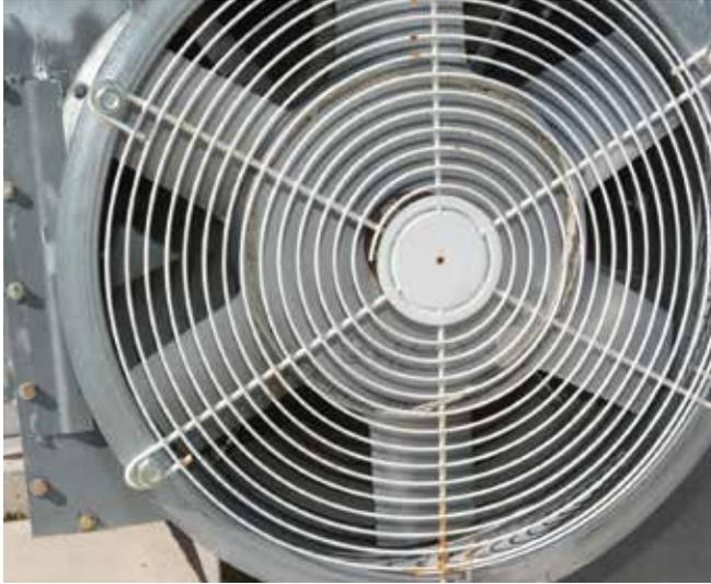
*Fig. 8-1. Axial flow fan.*
