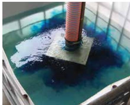
Figure 1A, left, shows what happens when colored liquid is added to the tank without the turbulence reduction device (TRD). Figure 1B with the TRD shows calmer water.
