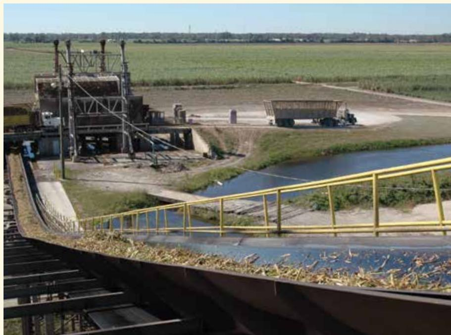
Harvested sugarcane is offloaded onto a conveyor that feeds the cane into the Lula Sugar Factory in Belle Rose for processing. Photo by Tobie Blanchard
