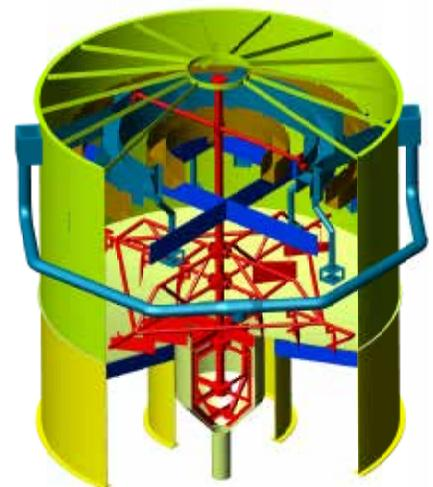
Figure 2, provided by Sterling Sugar Mill, shows how the TRD works in the clarifier design. The exit points of the pipes are supplied with TRDs that cancel momentum of the feed juice, thus eliminating turbulence eddies. For the past several seasons, these new clarifiers have been outperforming the existing design. Chromepion, an engineering company, purchased the exclusive license from the LSU AgCenter to market the invention worldwide.
