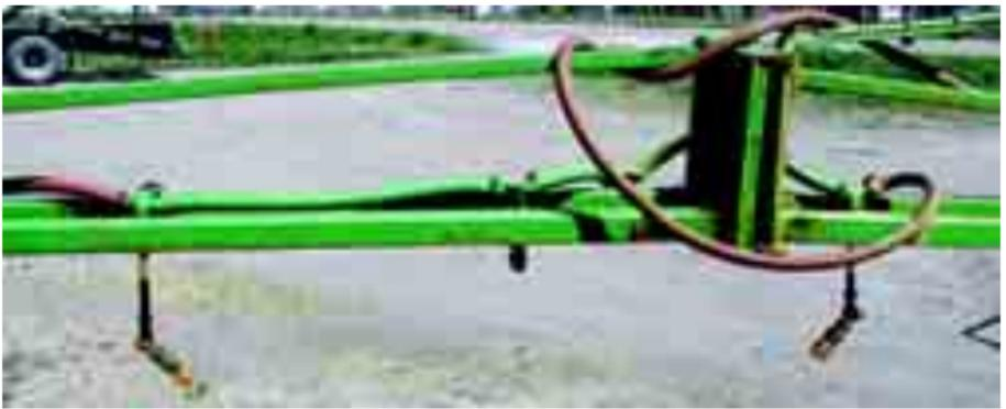
*Typical three nozzle per row arrangement for banded application of herbicide.*
