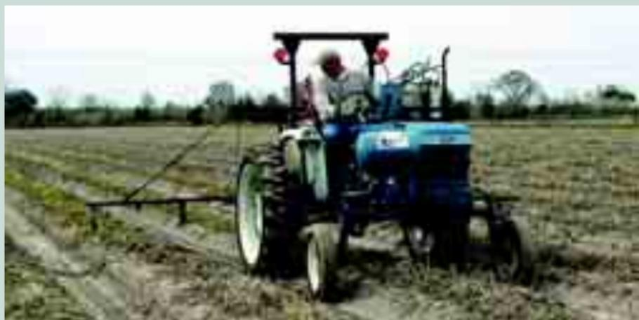
*Banded application of herbicide in March before sugarcane emergence using three nozzles per row.*
