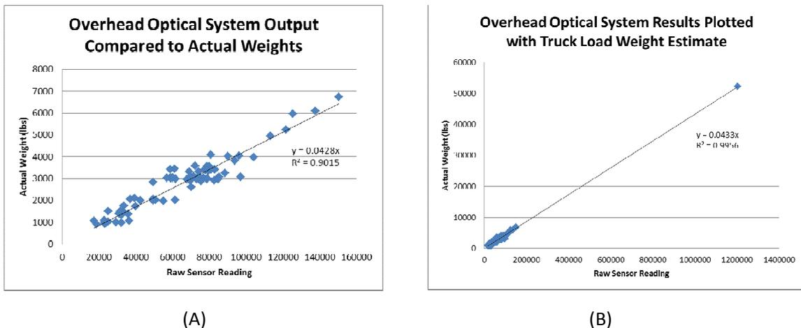
Figure 1: Result for overhead optical yield monitor and results plotted with truck load out weight (B).
