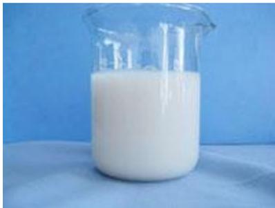
An **emulsion** is a mixture of droplets of one liquid in another liquid. Each ingredient keeps its unique properties and identity.
