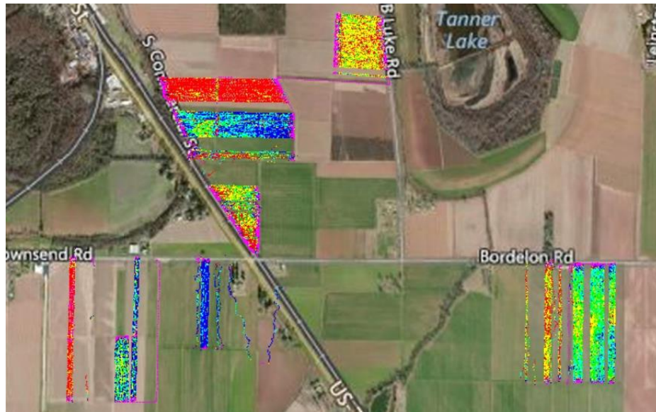
Figure 1: Calibration results from yield monitor for duty cycle (presence of billet per slat) and height and volume.
