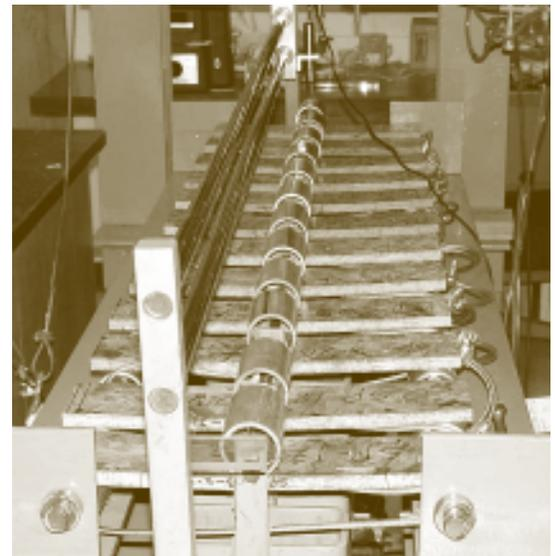
*Long-term structural testing of borate-modified oriented strandboard manufactured at LFPL.*
