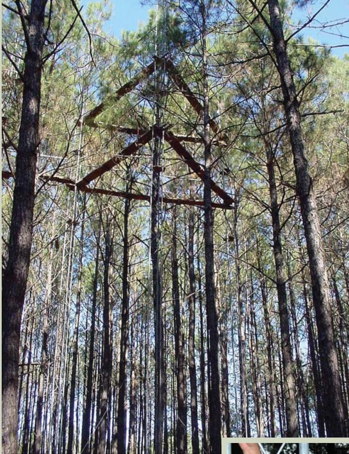
Above: Towers were built so the scientists can take measurements in the live canopy. The trees are about 40 to 50 feet high at this stage.
