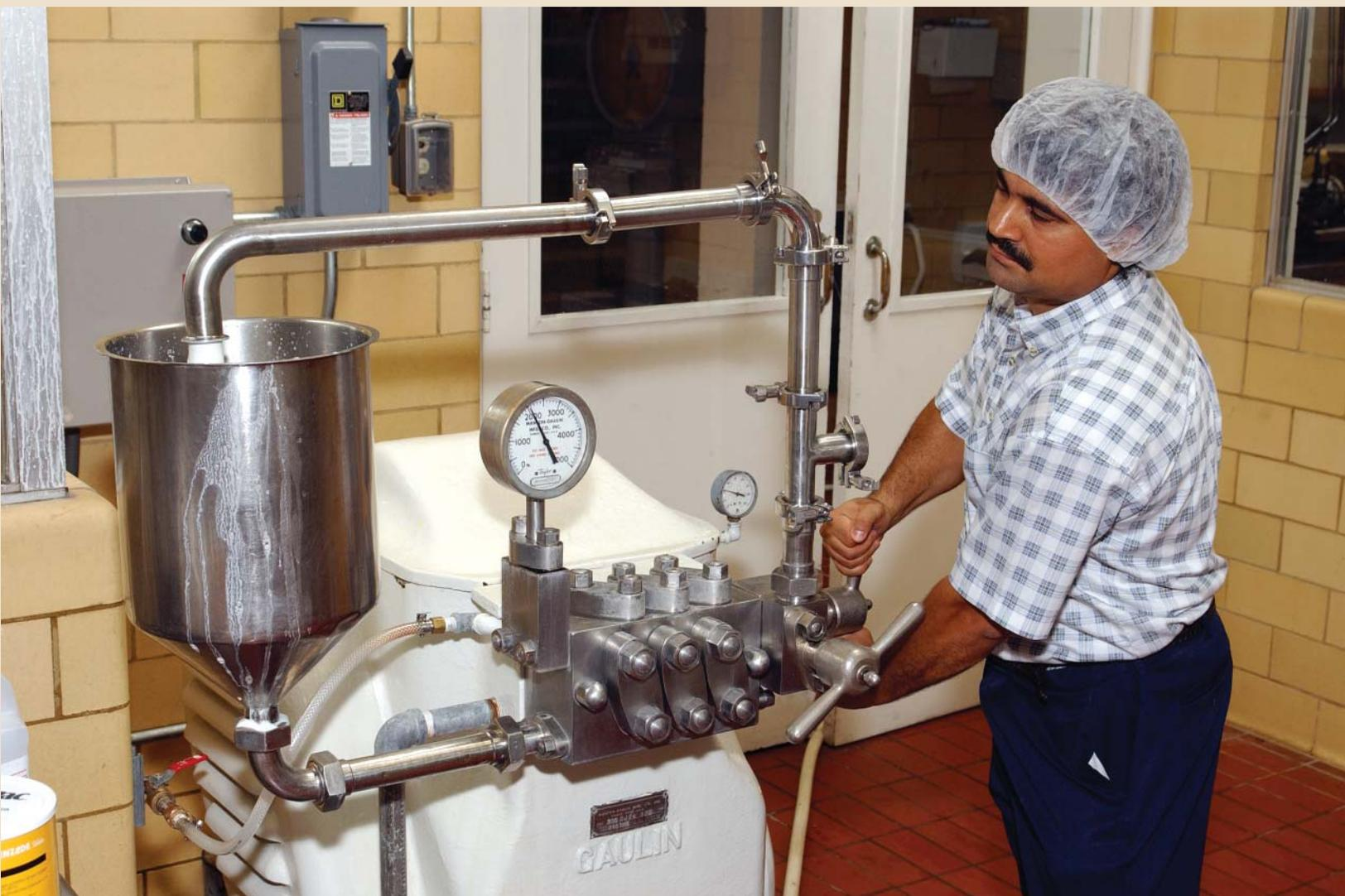
*Kayanush Aryana adjusts and monitors the pressure gauges of a homogenizing machine during the initial stages of making a healthier yogurt with folic acid.*
