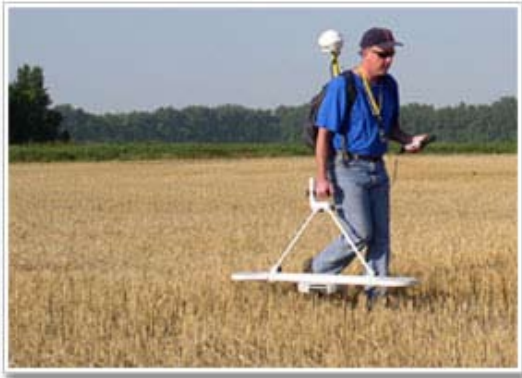
Figure 3. Electromagnetic induction measures soil electrical conductivity using noncontact sensors.
