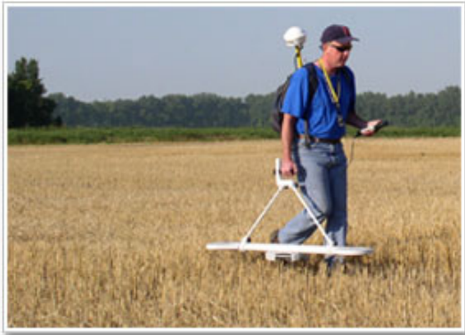
Figure 3. Electromagnetic induction measures soil electrical conductivity using noncontact sensors.
