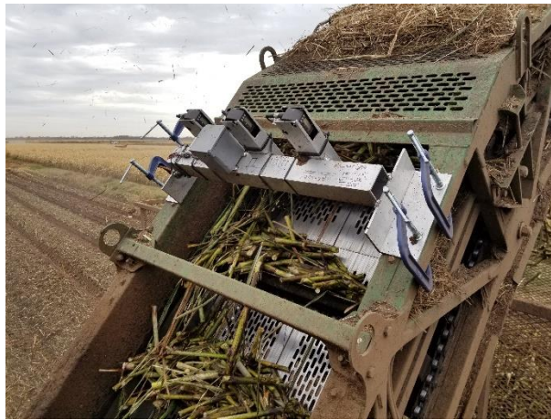
Figure 1: Newer overhead optical yield monitors composed of aluminum frame to help reduce weight and featuring built-in GPS and wireless capabilities.
