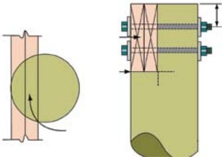
*Ideal beam to pile, post or column connection. Both bearing beams are fully supported with no over-cutting of the vertical support.*
