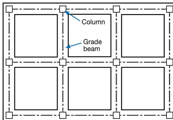
*Typical grade beam/column plan view. Spacing between columns should not exceed 14-feet if standard FEMA 550 foundation plans are to be used. Columns must be securely attached to the grade beam.*
