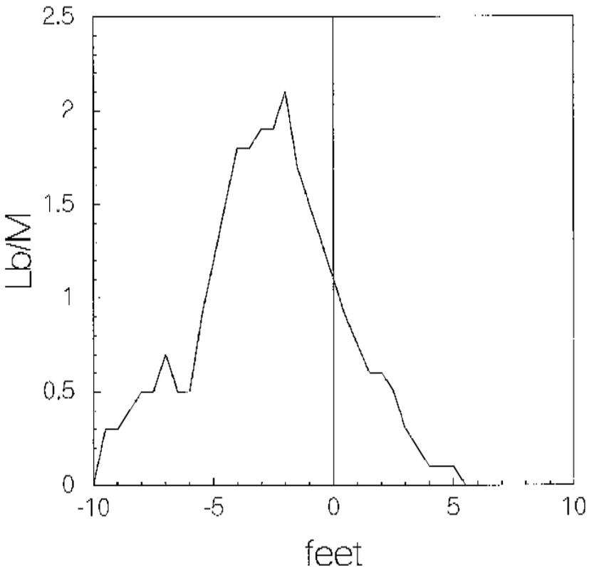
Figure 25. Typical skewed triangular pattern from some homeowner and semi-professional rotary spreaders.
