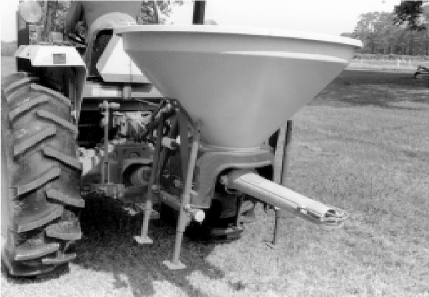
Figure 3. Example of pendulum broadcast spreader.
