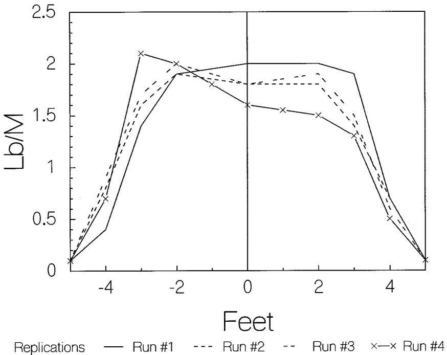
Figure 18. Pattern shift resulting from progressive buildup from methylene urea fertilizer in professional turf rotary spreader at 60% - 75% relative humidity.
