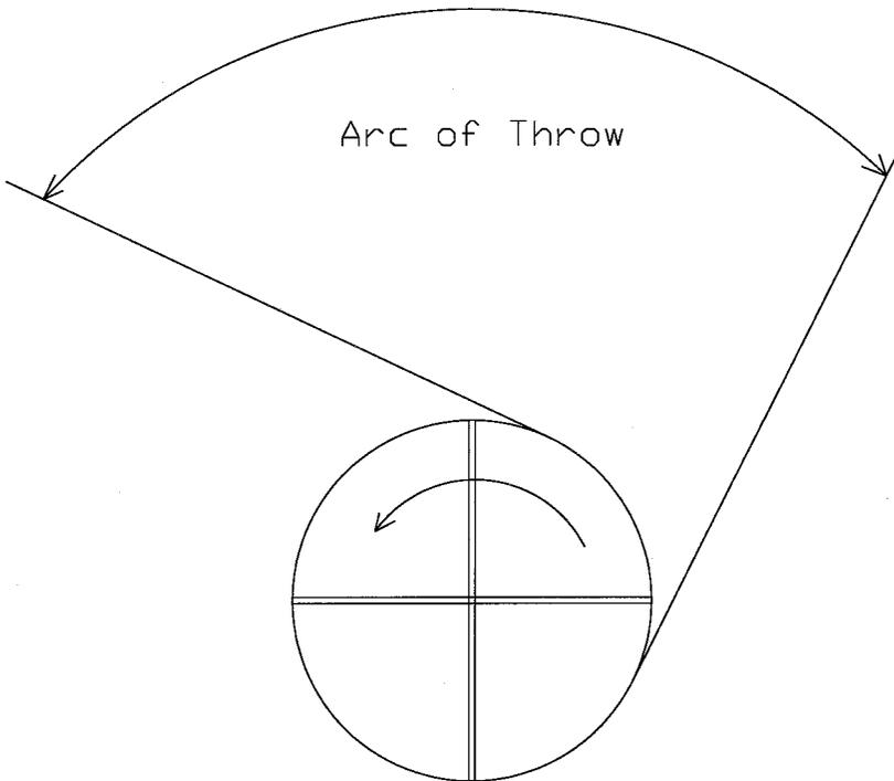
Figure 7. Illustration of material leaving spreader impeller in an arc.
