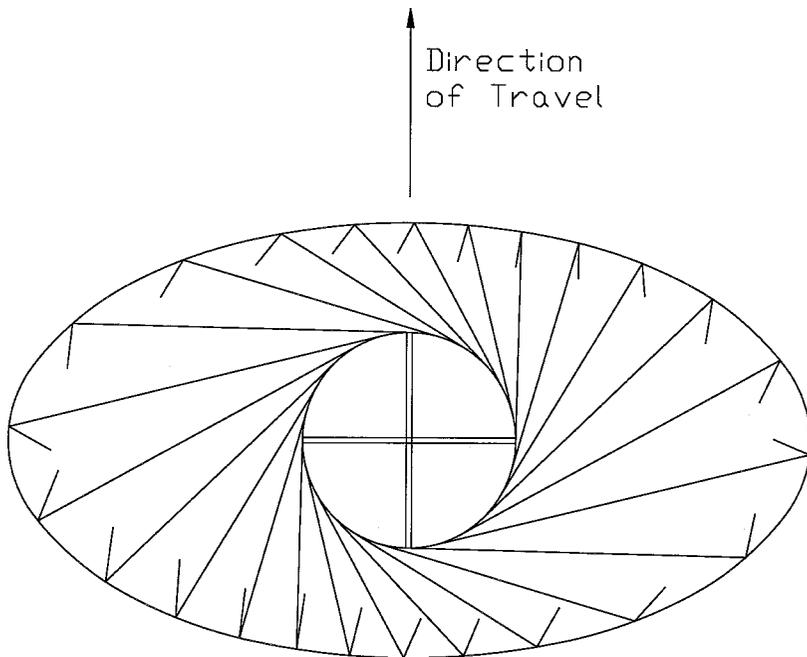
Figure 9. Trajectory of granules in elliptical shroud.
