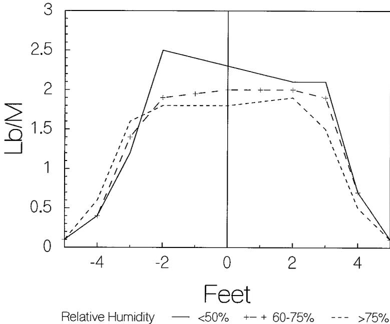
Figure 17. Pattern shift with increasing ambient humidity with methylene urea fertilizer in professional turf rotary.
