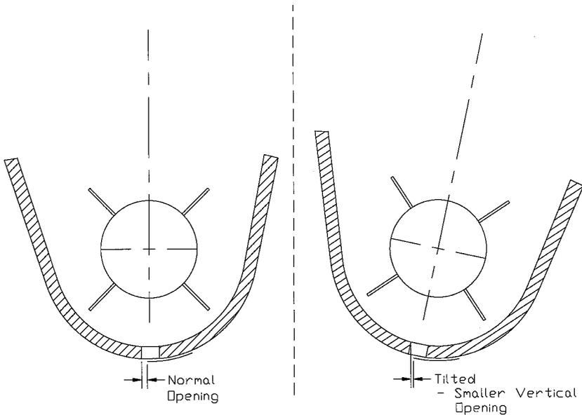
Figure 10. Effect of angle on thick hopper bottom: a) normal angle, b) spreader tilted back 12°.
