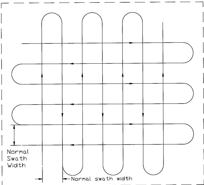
Figure 23. Right-angle method of spreader pattern correction.
