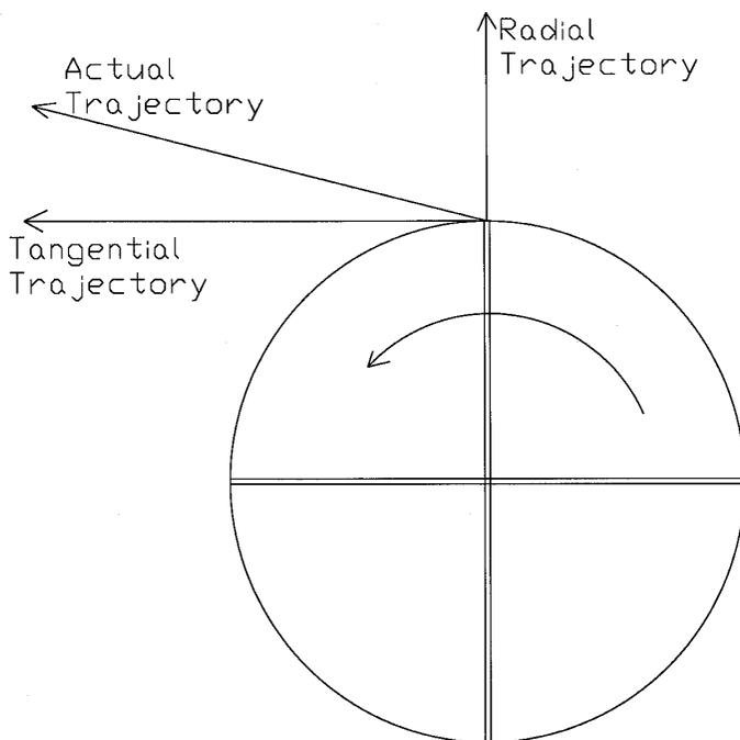
Figure 6. Typical trajectory of a granule leaving a spreader impeller.
