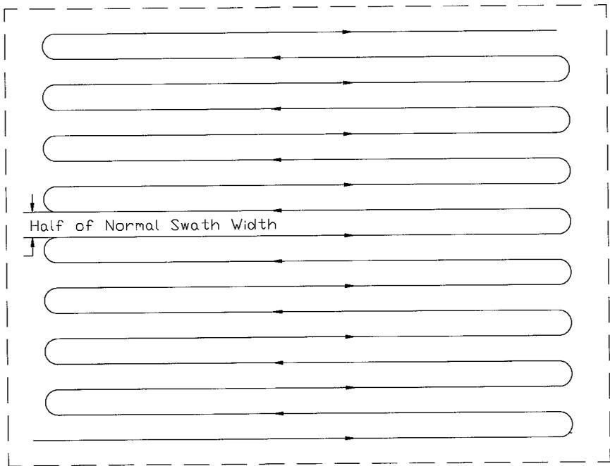
Figure 24. Half-width method of spreader pattern correction.
