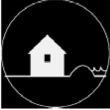
**A levee is a barrier that holds water away from the building. It can protect your home from flooding as well as from the force of water, scour at the foundation and impacts of floating debris.**
