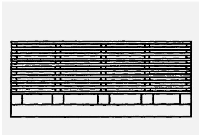
**Figure 13.** A properly stacked pile of lumber has stickers of equal thickness that are vertically aligned. The normal distance between stickers and braces is 18-24 inches.
