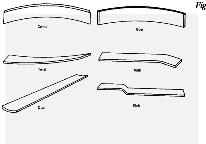
**Figure 5.** Drying defects that can occur in improperly seasoned lumber.
