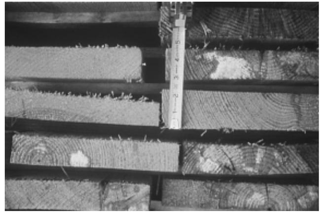
**Figure 14.** These southern pine boards are of uneven thickness. The board that is too thin was miscut and should have been culled or at least sorted out before stacking.
