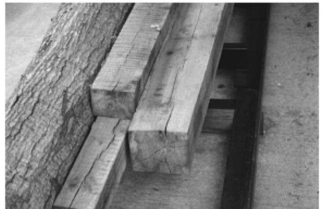
**Figure 16.** End checks in cants caused by rapid drying and sun exposure. End checks that develop in logs will also be present in the lumber that is sawn.
