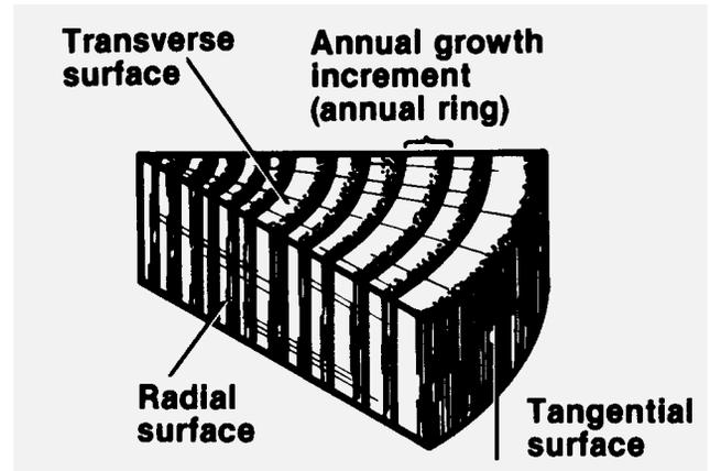
**Figure 2.** The three primary surfaces of wood. Dimensional movement is unique in each of these three planes. (Source: USDA Forest Products Laboratory 1987)
