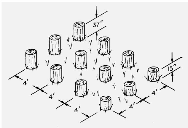
**Figure 7a.** A good foundation is needed for correct stacking and good seasoning. Use treated wood, steel or concrete.
