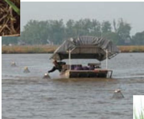
*Harvesting crawfish with an aluminum boat equipped with a rear wheel hydraulic unit and foot operated steering controls. (photo by*
