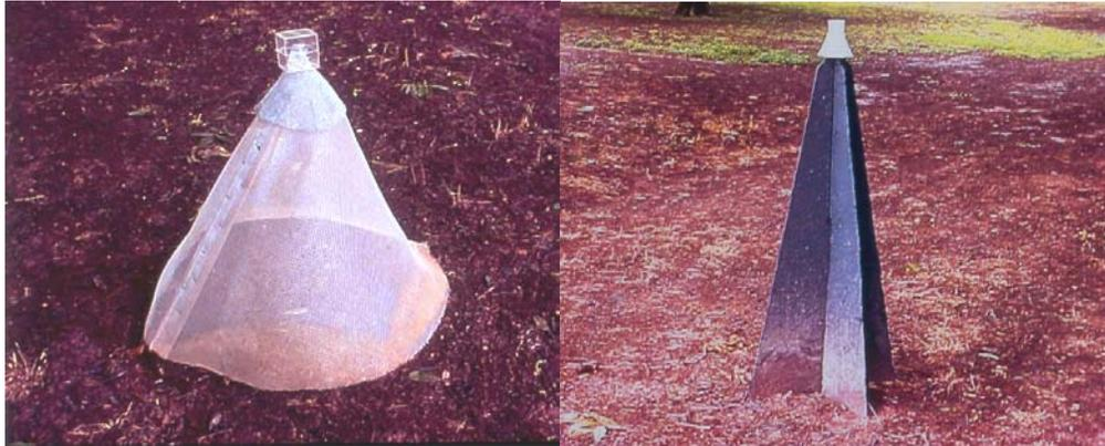
Figure 4. Wire cone emergence trap.
