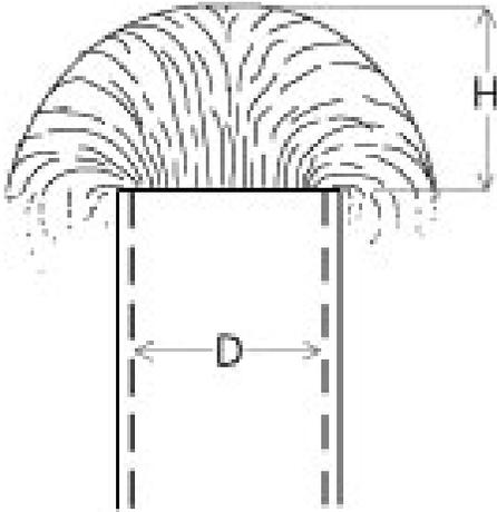
Figure 9. Flow from a vertical pipe or casing.
