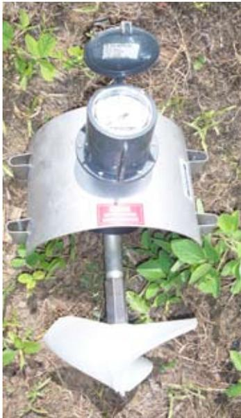
Figure 1. Propeller flow meter.
