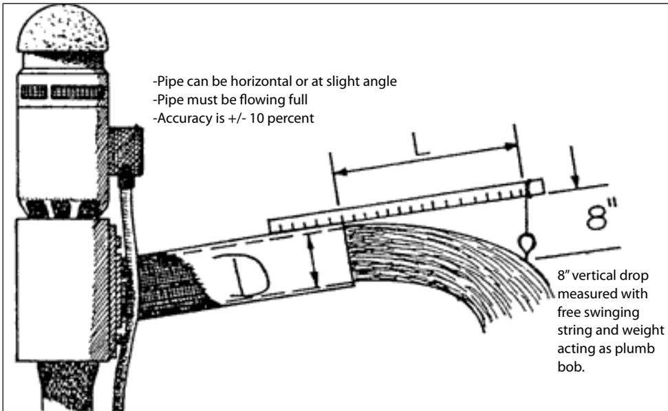
Figure 7. Measuring a pump flow using a Plumb-Bob.
