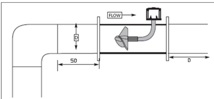
Figure 6. Proper placement of flowmeter on an irrigation system.
