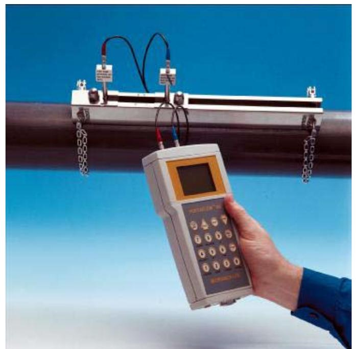
Figure 4. Ultrasonic flow meter.
