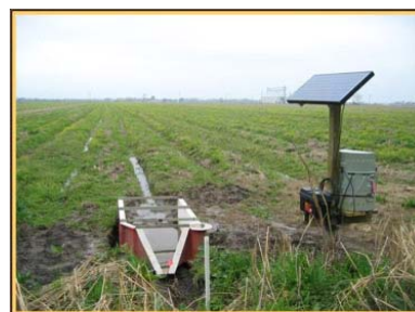
Water capture and sampling devices consisted of flumes and automated samplers energized by solar-powered batteries.
