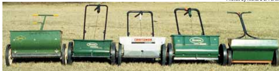
Figure 1. Spreaders used for the drop spreader metering uniformity study: Gandy professional (steel), Scotts AccuGreen 1000 (plastic), Republic/Sears/K-Mart EZ Drop (plastic), Scotts AccuGreen 3000 (plastic), obsolete Scotts PF-1 (steel).
