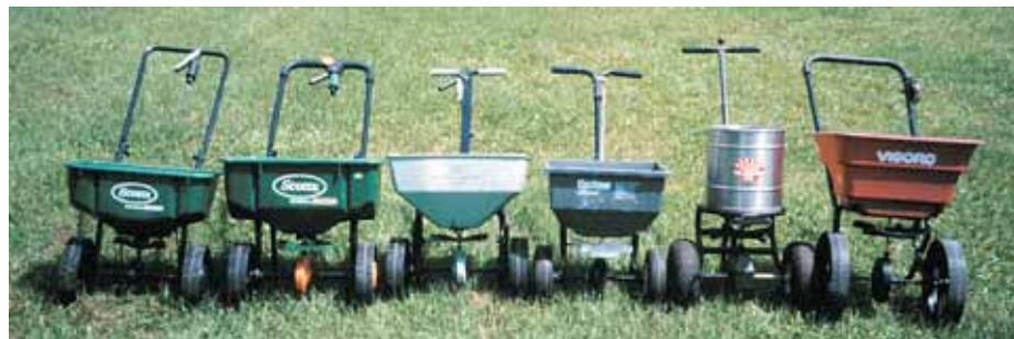
Figure 2. Spreaders used for the rotary spreader pattern study: Scotts Speedy Green 1000, Scotts Speedy Green 3000, Republic/Sears/K-Mart EZ Broadcast, Cyclone, Spyker and Vigoro.
