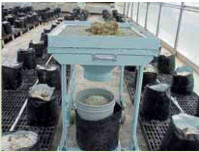
Figure 1. A movable hopper with a wire mesh screen is used for sifting the perlite.
