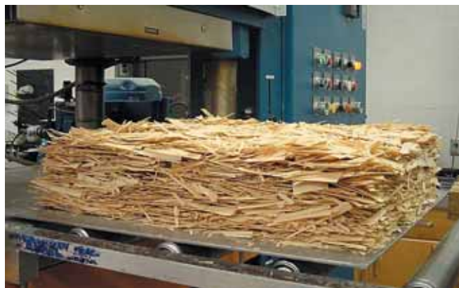
Flake mats with resin- and borate-coated southern pine flakes ready to be hot-pressed.
