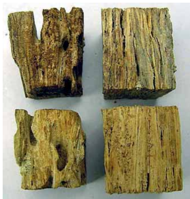
A comparison of damaged (top) and undamaged test samples.
