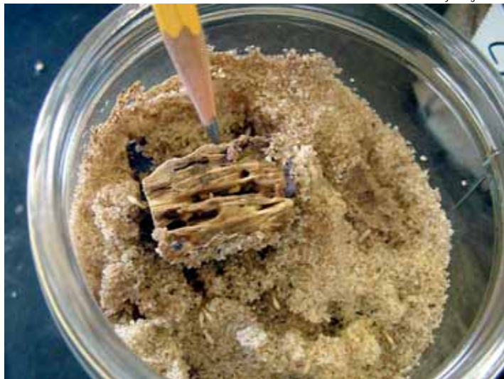
An oriented strandboard sample (southern pine) in a test bottle with Formosan subterranean termites tunneling through the sample.
