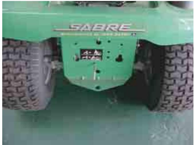
Figure 14. Drawbar hitch on lawn tractor.
