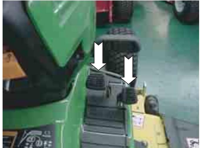
Figure 9. Pedals to operate hydrostatic transmission.
