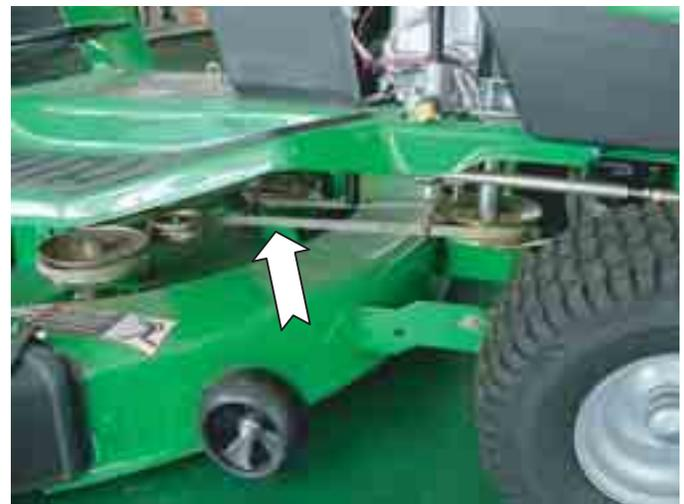
Figure 10. Belt drive to mower deck.
