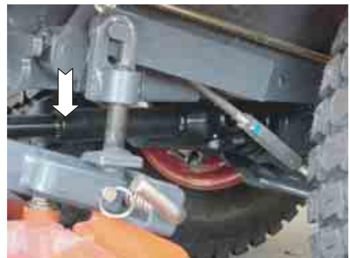
Figure 11. Shaft drive to mower deck.
