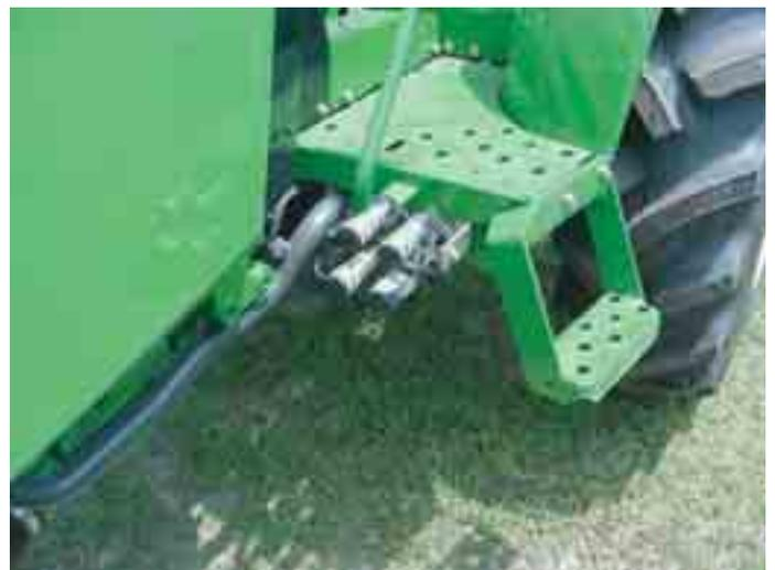
Figure 13. Remote hydraulic outlets on tractor.
