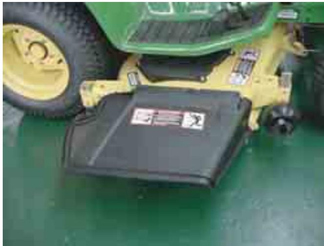
Figure 18. Discharge chute in place.
