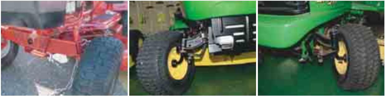
Figure 17. Formed and welded front axle on cheap tractor on the left; cast iron front axle on small lawn tractor in the center, forged front axle on higher quality tractor on the right.
