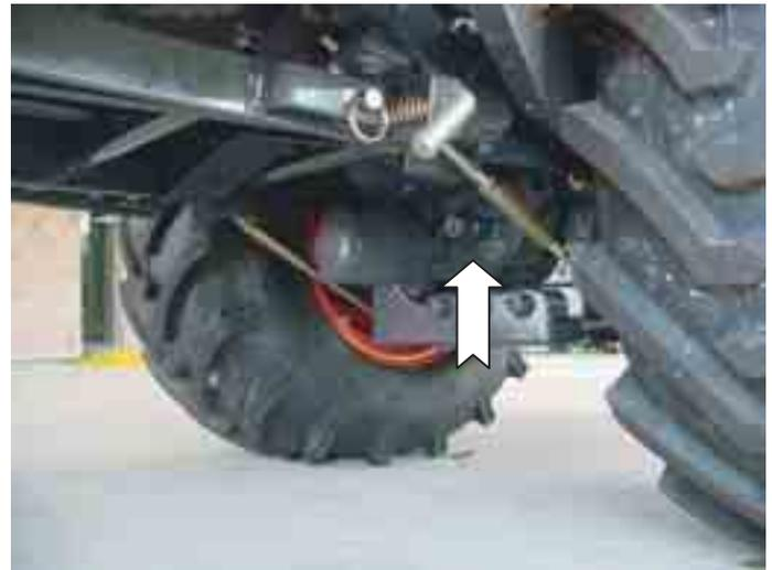
Figure 12. Mid-mount PTO shaft.
