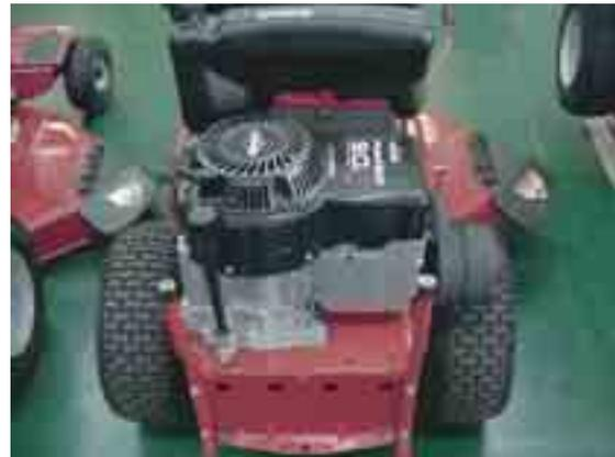
Figure 4. Vertical-shaft engine.
