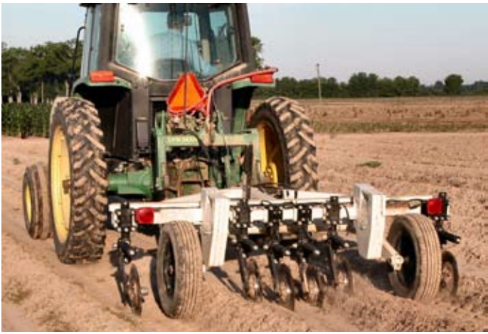
Figure 2. The Veris 3100 Soil EC Mapping System collecting data in a field.
