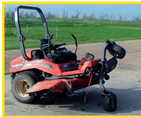
Figure 14. Leg at front of ZTR mower to tilt entire machine for deck service.
