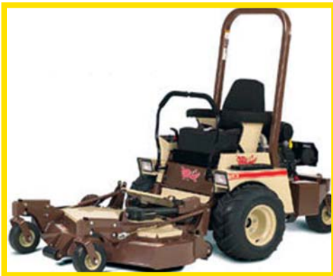
Figure 11. ZTR mowers with front-mount decks can have a very low center of gravity, hanging obstacles since the area over the deck is clear. Mid-mount decks generally have some clear overhang on the sides and front, but not as much as front-mount decks.
