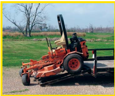
Figure 25. Mid-mount ZTR mowers should be backed up ramps and slopes to avoid overturns.
