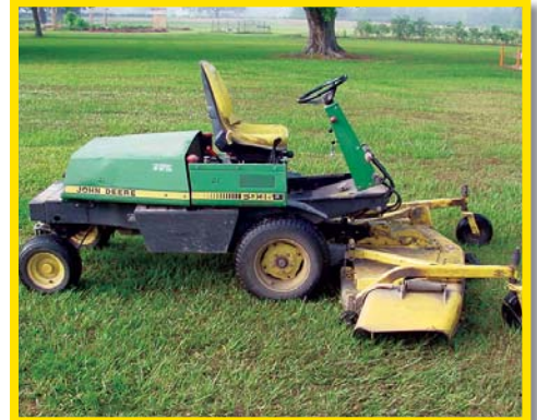
Figure 10. Front mount deck on mower with steerable rear wheels (not a ZTR mower)
