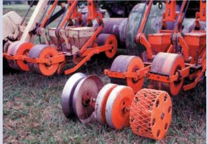
On the left is a standard smooth presswheel with a paired arm covering device. At right are three other types of presswheels, left to right, the concave split, the flat split and the cage.
