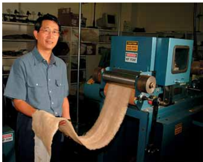
Yan Chen holds the fiber web that has been needle-punched for further compaction.
