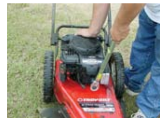
Figure 16. Use a torque wrench to tighten the spark plug to avoid stripping threads.
