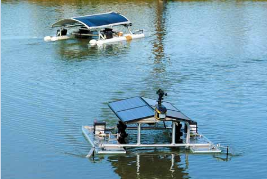
These two prototypes of the scarebots are each about 4 feet by 4 feet in area and about 18 inches high. The LSU AgCenter engineers are also working on larger models to be used in lakes and reservoirs.
