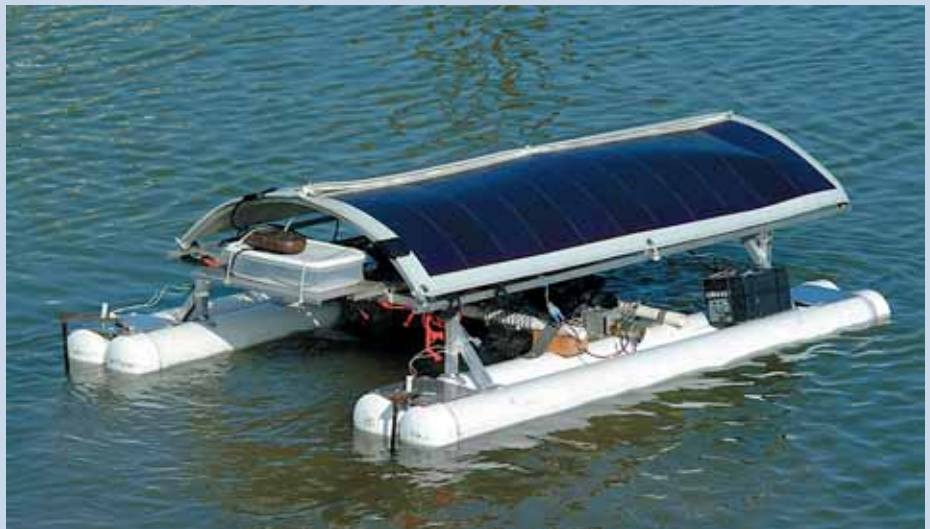
This is one of the first models created by the LSU AgCenter engineers. The boats are propelled by paddle wheels and reach top speeds of 5 to 7 miles per hour.
