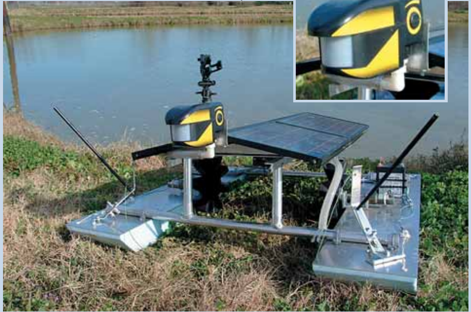
The thin metal rods on each side contain shore sensors that keep the boat from running aground. The painted head sticking up from the boat contains an infrared sensor to detect motion, which triggers a water cannon that annoys and drives away the birds.
