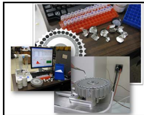
The N-combustion analyzer used to measure total crude protein content of rice grain for screening purposes.
