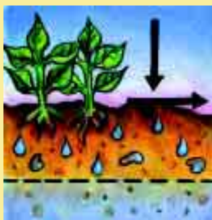
The water table separates the unsaturated zone from the saturated zone (groundwater)
