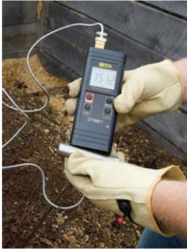
Figure 1. One example of a temperature probe. (Notice the temperature of 151°F.)
