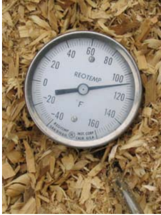
Figure 2. An example of a dial type thermometer. (This pile needs to warm up.)
