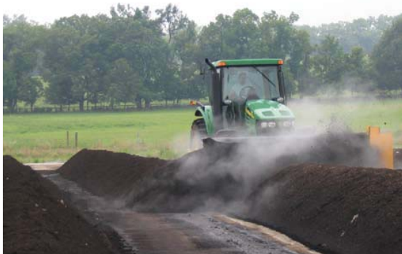
Figure 6. Turning compost with a mechanical turner.
